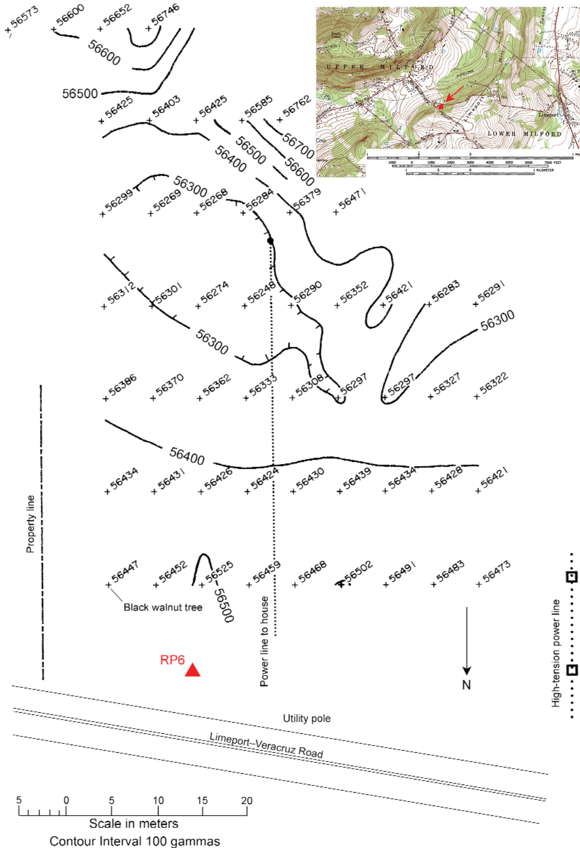
Figure 64. Contour map of total magnetic flux in gammas at the Limeport Road anomaly, Upper Milford Township, Lehigh County. Allentown East 7.5-minute quadrangle; 40°30'37"N, 75°28'15"W.
